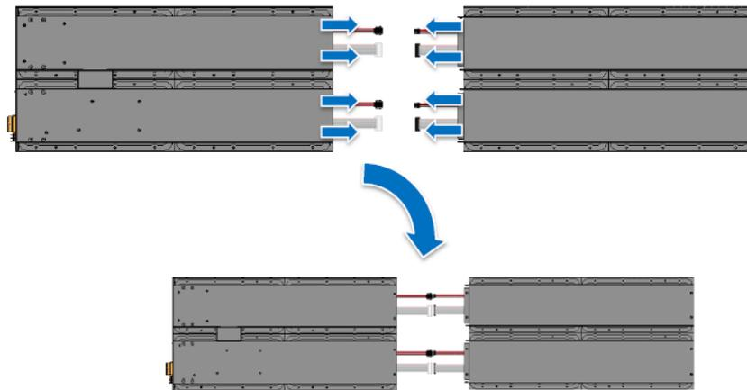
3. Attach the modules and fasten the modules together with 6/8 supplied screws
